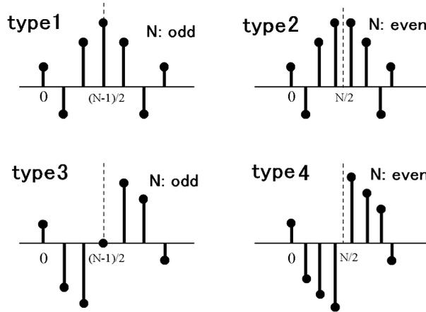
Figure 1: Four types of FIR filter
